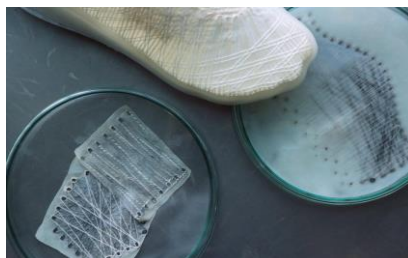
Figure 1. Biodesigner Jen Keane has developed an interesting "microbial weaving" process by manipulating the growth of k. rhaeticus , a type of bacteria typically found in kombucha tea. The resulting material, a synthetic fiber, is stronger than steel and more resistant than Kevlar © Vita Larvo, Retrieved from: https://www.lifegate.com/biomaterials-design-future [7].
