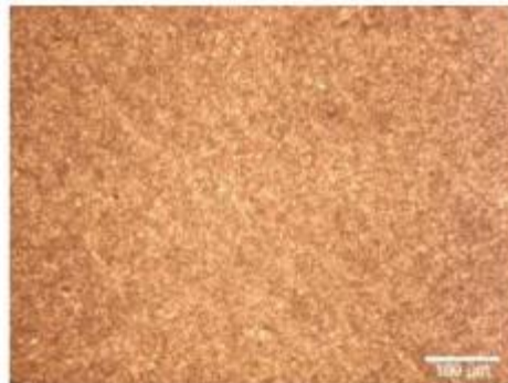
Figure 4. Optical micrography of the broken ball stud. 3% Nital. The structure is tempered martensite.
