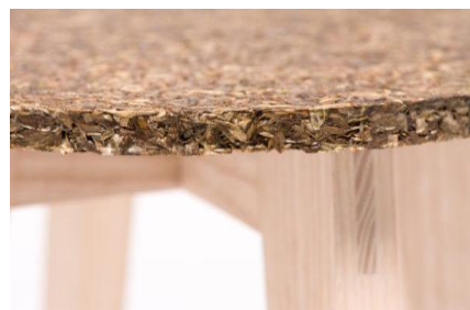
Figure 5. Zostera Stool , Figure showing seating material thickness 1cm. Carolin Pertsch (2017, January 27). Zostera Stool: Sitting on washed-up seagrass . Retrieved from https://materialdistrict.com/article/zostera-stool-sitting-washed-up-seagrass/ [9].
