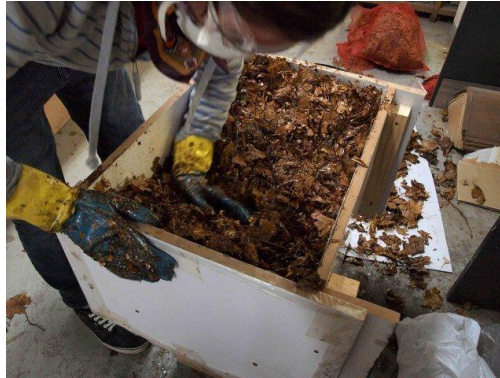
Figure 10. Process of pressing dried leaves with resin into the mould. Retrieved from, http://simonkern.sk/object/beleaf-chair-16.html [12].
