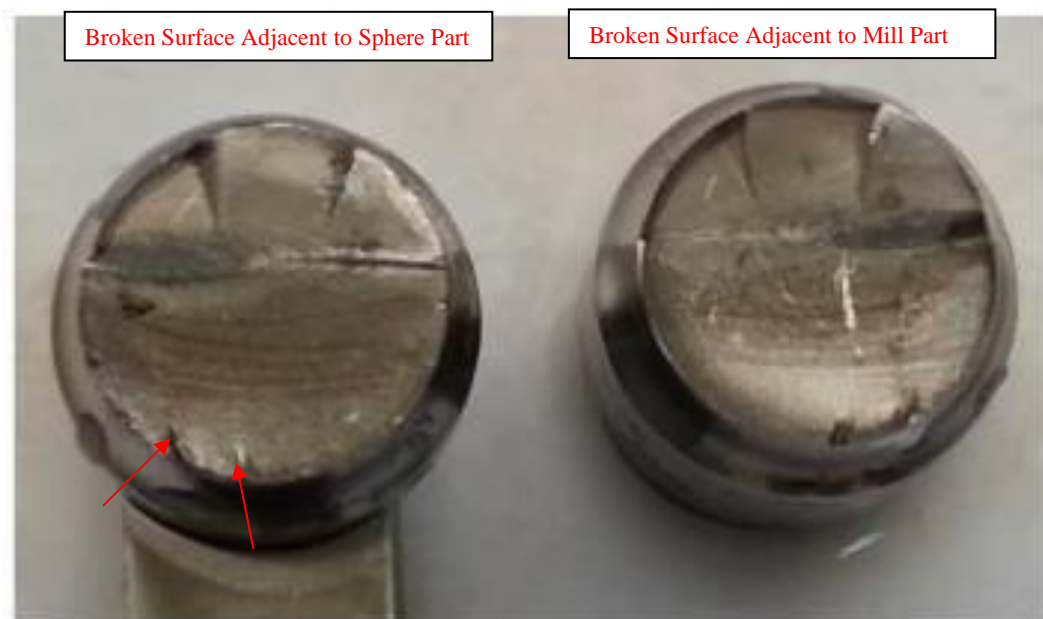
Figure 3. Broken surfaces of ball stud part. Typical bending fatigue failure image.
