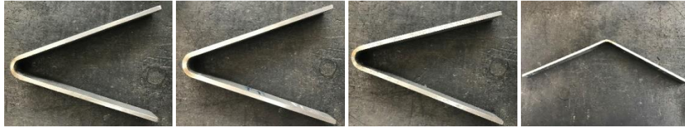
Figure 9. Macrographs showing the surface and root bend specimens extracted from: (a) lower heat input joint and (b) higher heat input joint. Note that no cracking occurred in any of the specimens.
