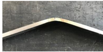
Figure 10. Macrograph showing the failure location in root bend specimens extracted from the higher heat input joint. Note that failure takes place in the coarse grained HAZ (CGHAZ) region.
