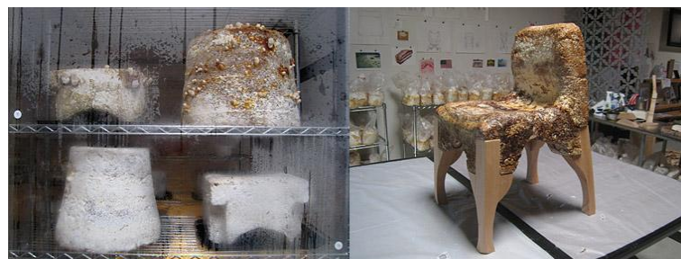
Figure 3. Showing Stages of mycelium on cellulose and development of fungi, Exhibition at Espace Foundation. Retrieved from http://thisisalive.com/yamanaka-furniture/ (2012) [8].
