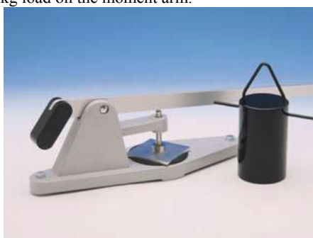
Figure 2. WIRA instruments - prolonged heavy static loading test device [4]
