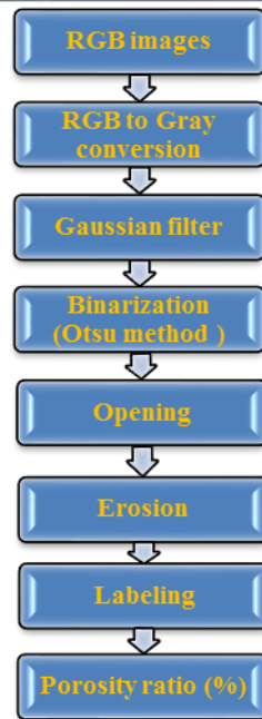
Figure 1. Porosity and pore labeling algorithm
