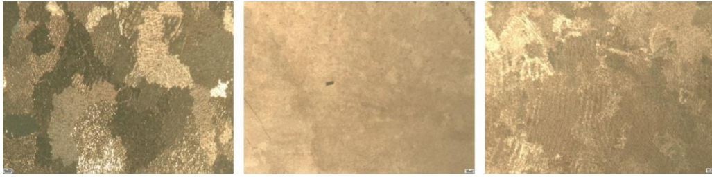
Figure 2. Stereo microscope images of the samples after immersion tests; in HCl (left), in NaCl (middle), in H 2 SO 4 (right) solutions
