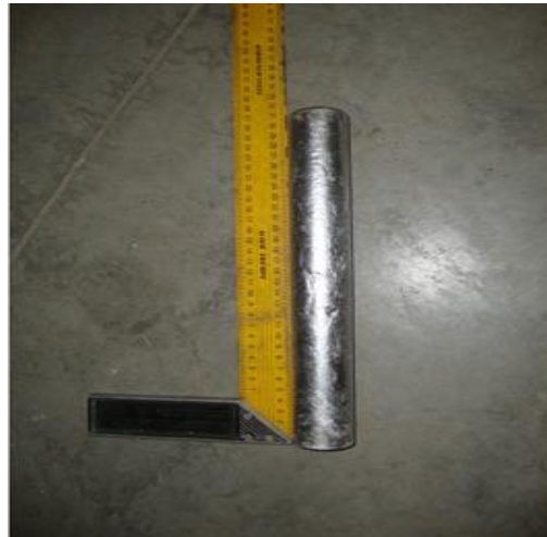
Figure 1. The macrograph of as cast A380 alloy billet
