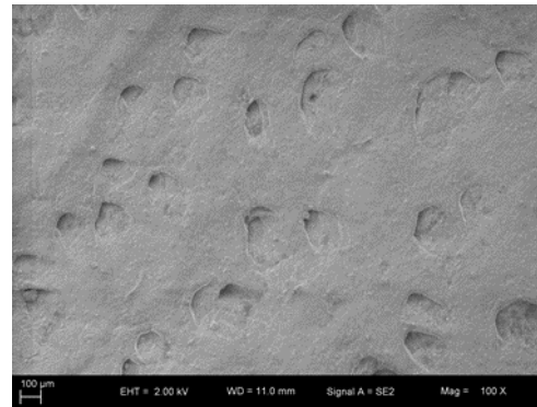
Figure 6. (b) SEM image of 14% Leather Samples in 100 \mu\text{m} Magnification
