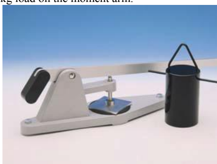
Figure 2. WIRA instruments - prolonged heavy static loading test device [4]
