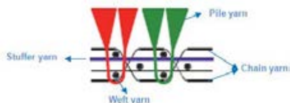
Figure 1. 2/3 V weave construction [16,17]
