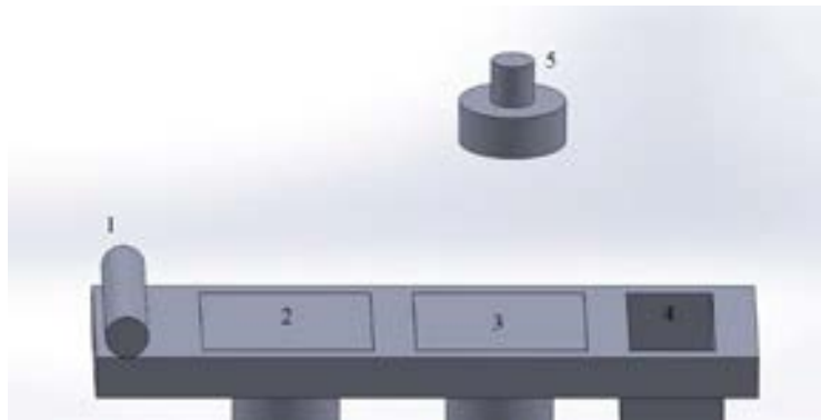
Figure 2. Selective Laser Melting Hardware (1. Roller, 2 Powder bed, 3 Process bed, 4 powder removal system, 5 Laser system.)
