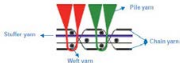
Figure 1. 2/3 V weave construction [16,17]
