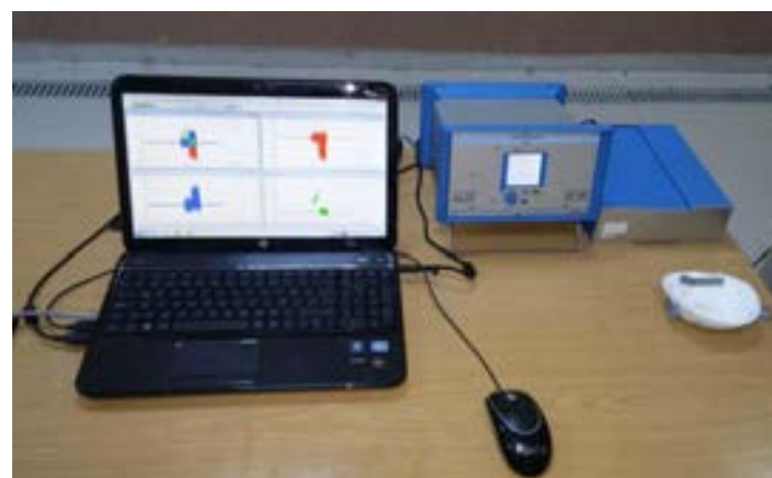
Figure 3. Thrust force measurement instruments
