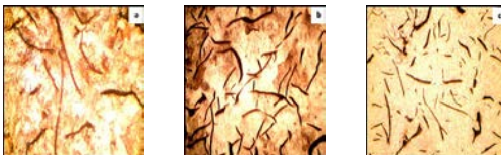
Figure 3: Microstructure drawings of specimens of lamellar graphite cast iron produced at a casting temperature of 1350°C (x200) a) GLJ-A b) GLJ-B c) GLJ-C
