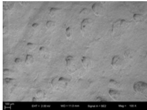
Figure 6. (b) SEM image of 14% Leather Samples in 100 μm Magnification
