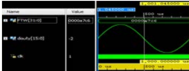
Figure 25. The Generated 1 kHz sine wave (clk =100 MHz)
