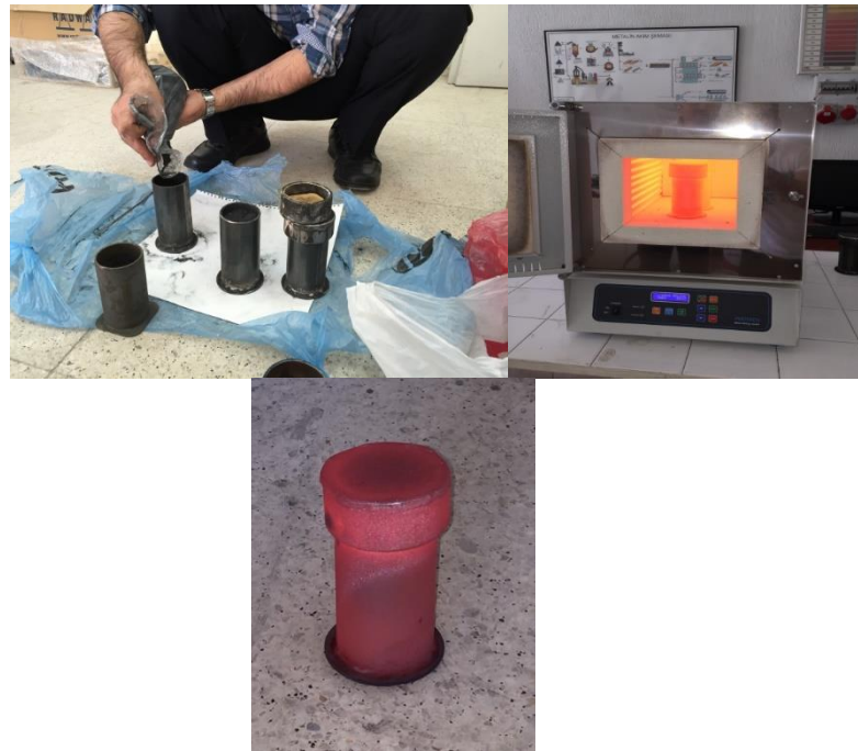
Figure 1. Boriding heat treatment of Tungsten alloys
