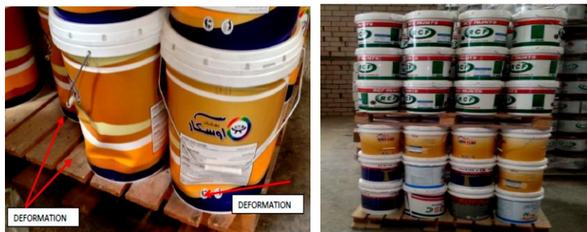
Figure 7. Pails stacking matrix and the visible deformation.
