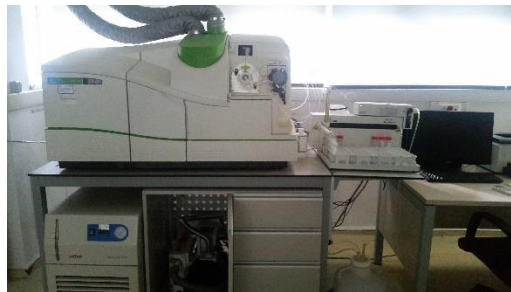
Figure 26. Nexion 300D model ICP-MS
