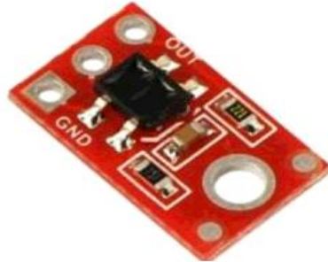
Figure 4. QTR-1A Infrared Sensor
