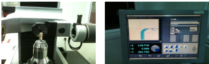
Figure 22. 3D laser scanning radius measurements (Operation is on the left, calculation the results is on the right)
