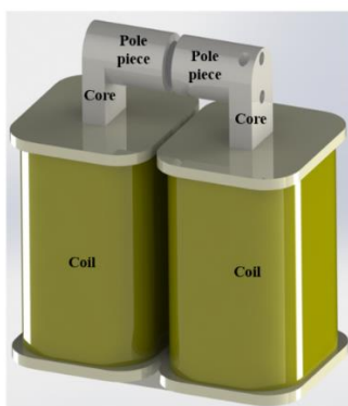
Fig. 3 (a) Modeling of electromagnet
