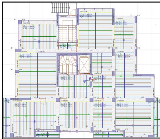
Figure 5. Formwork plan of building made with hollow-tile floor slab
