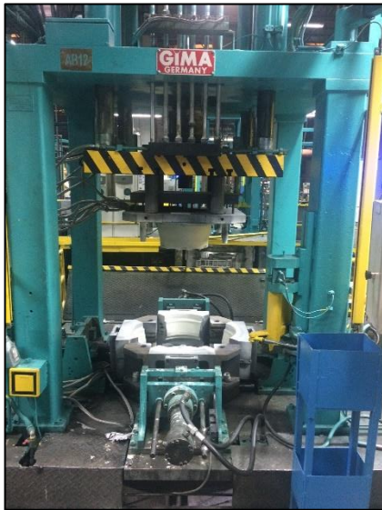
Figure 14. (a) LPDC (Low Pressure Die Casting) method
