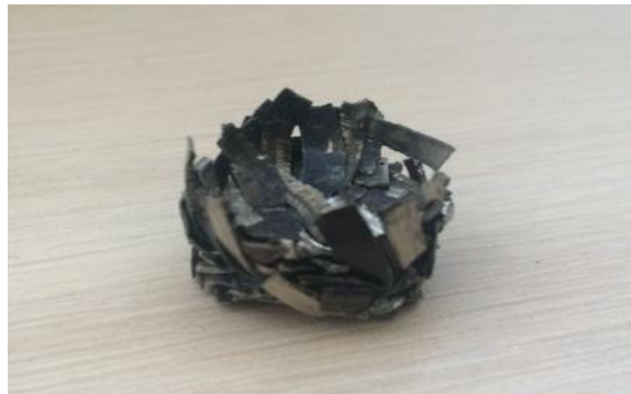
Figure 1. Porous one-piece preform made by 304 SS and CP-Ti sawdusts
