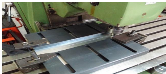
Figure 1. The milling machine used for FSW process
