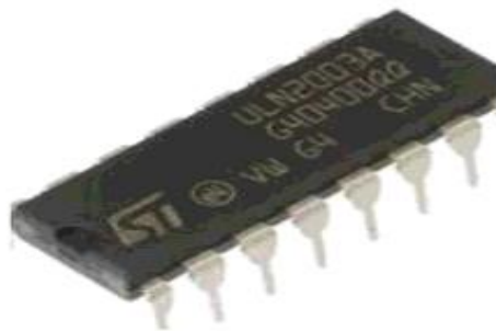
Figure 2. Step Motor Driver Integrated Circuit
