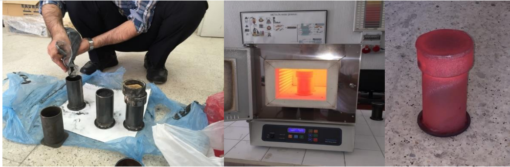
Figure 1. Boriding heat treatment of Tungsten
