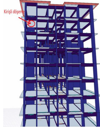
Figure 4. View of beam-slab
