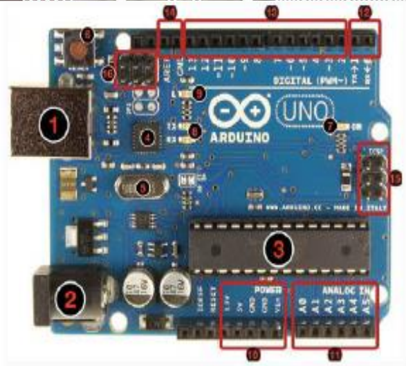
Figure 3. Arduino Uno Circuit
