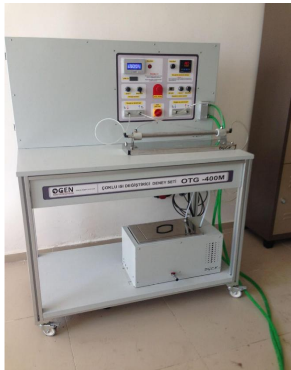
Figure 2– Double pipe heat exchanger experimental setup
