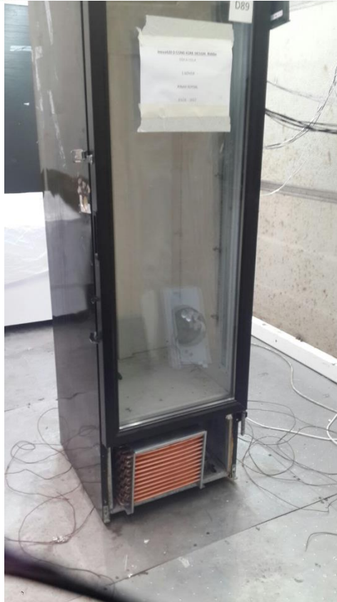
Figure 2 – Vapor compression refrigeration system used in the experiment with condenser made of copper circular tubes
