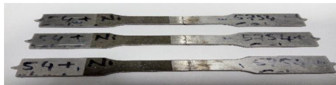
Figure 12. Tensile test of coated and welded AA5754 aluminum alloy (ASTM E8M-04)
