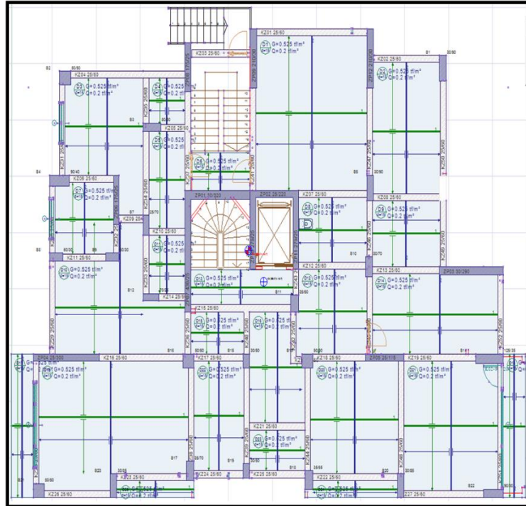
Figure 2. Formwork plan of the building made of beam-slab
