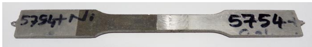
Figure 6. Standard tensile test samples (ASTM E8M-04 ) of the welded sheet
