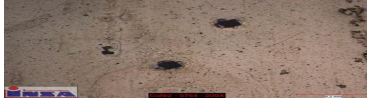
Figure 9. OM micrograph of Ni-Cu particles observed in the stir zone of an AA5754 aluminum alloy welded by FSW
