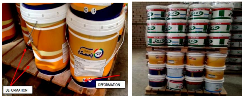
Figure 7. Pails stacking matrix and the visible deformation.
