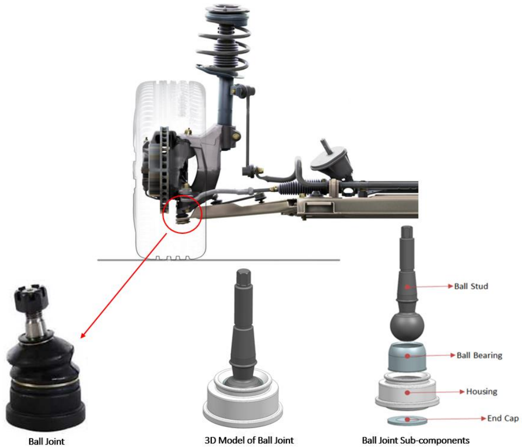
Figure 1. An assembly of ball joint in front suspension system
