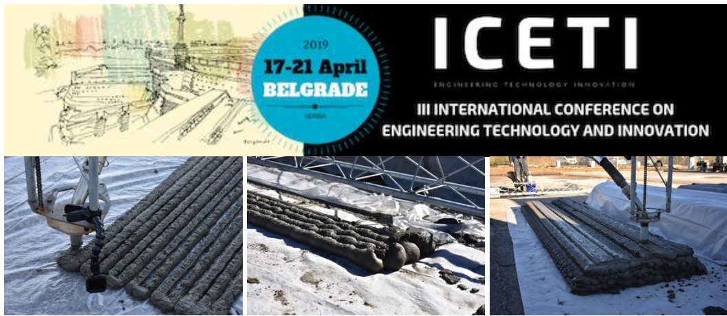
Figure 12. (a) Original 3.2cm nozzle (b) No nozzle (c) New 5.1cm nozzle
