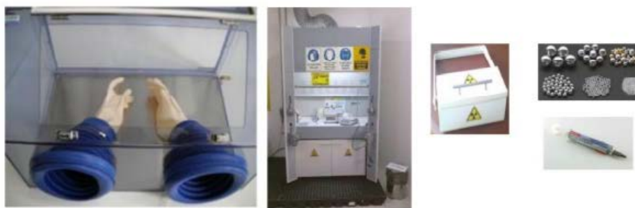
Figure 8. Glovebox, Lead Cell Fume Hood, Lead Carrying Container, Balls, Injector (Keles, 2021)
