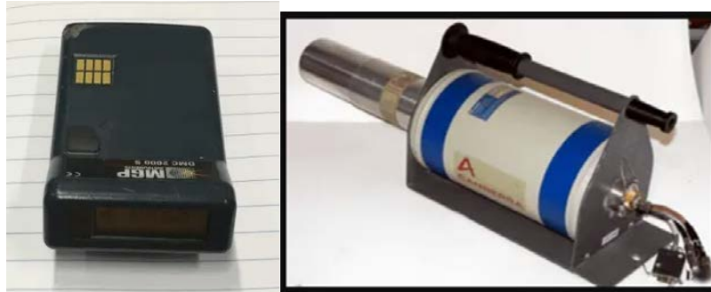
Figure 2. Electronic personal dosimeter and detector-germanium (Epsilon, 2021)
