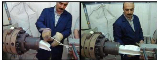
Figure 8. Extruded Material which connects to Calibration Stage
