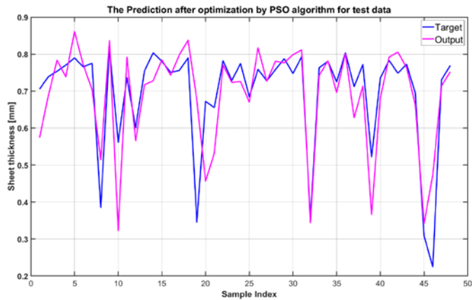
Figure 6. Comparison of the predictions output and target output after optimization by PSO for test data
